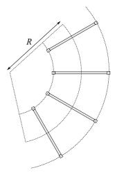
Taking into account that  $\varphi = \varphi_0 + \omega_0 t$  (where  $\varphi_0$  is the initial angle between the rod and the steepest line), the equation of motion is analogous to the differential equation of a harmonic oscillator. So the magnitude of the velocity of the center of the rod as the function of time is given by
