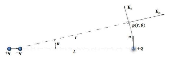
Figure 3: The system analyzed in Part 2. (Direction of the vector  $\mathbf{E}_{n}$  and  $\mathbf{E}_{t}$  could be wrong)
